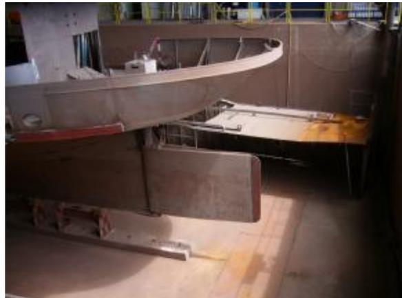
The “electronic” display telling the machine operator what to do. And the raw rudder in the dry dock, being prepared for fine painting.
